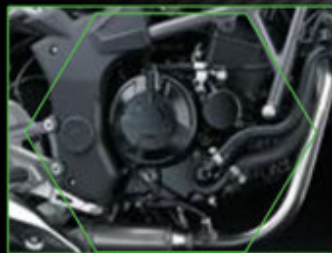
249 cm3 liquid-cooled, 4-stroke Single
